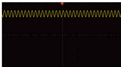
DC+AC Vdc=50V, sine ripple Vac=5V, frequency 1000Hz
