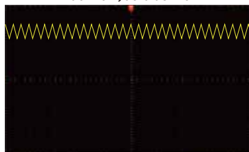
DC+AC Vdc=50V, triangle ripple Vac=5V, frequency 1000Hz
