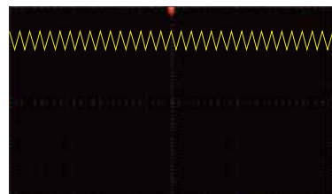
DC+AC Vdc=50V, triangle ripple Vac=5V, frequency 1000Hz
