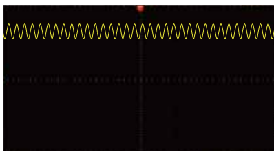
DC+AC Vdc=50V, sine ripple Vac=5V, frequency 1000Hz
