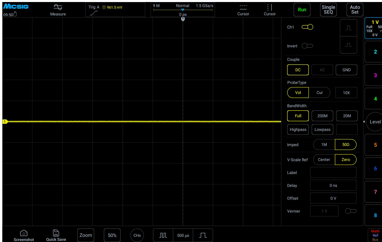
Figure 5-18 Channel input impedance
