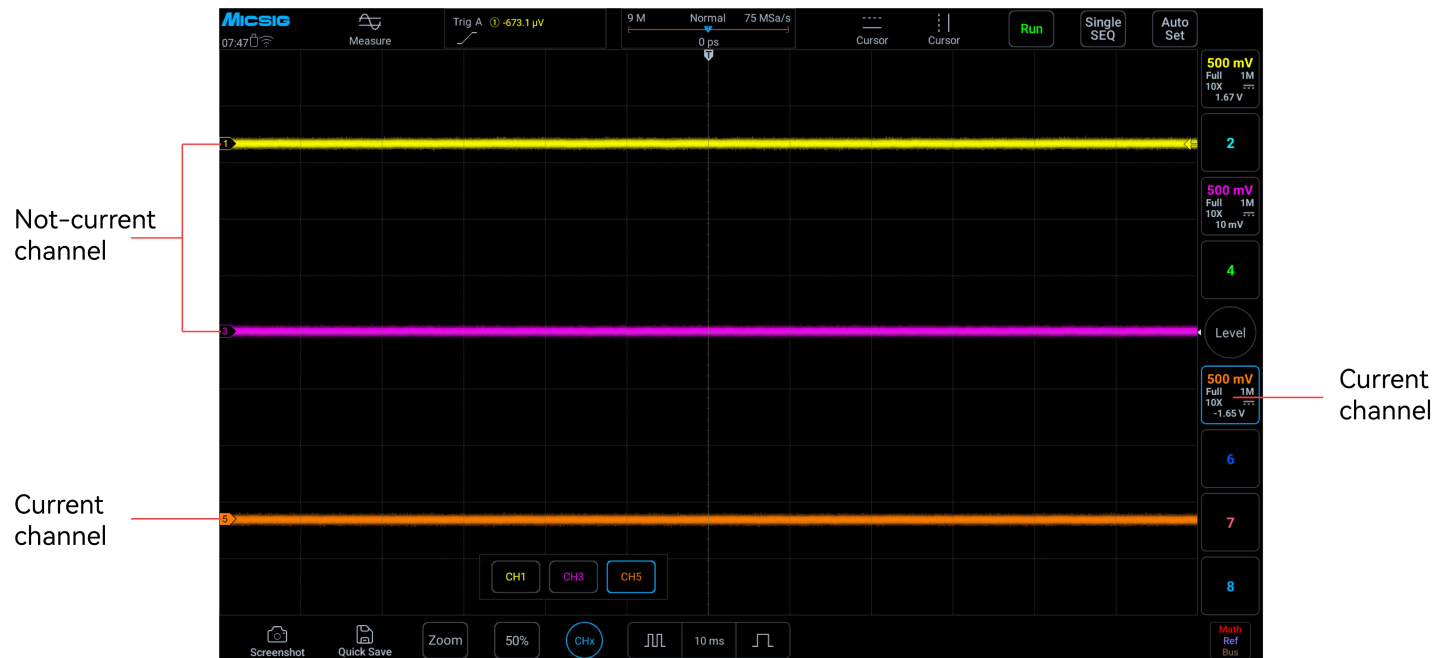
Figure 5-2 Current Channel and Non-Current Channel
