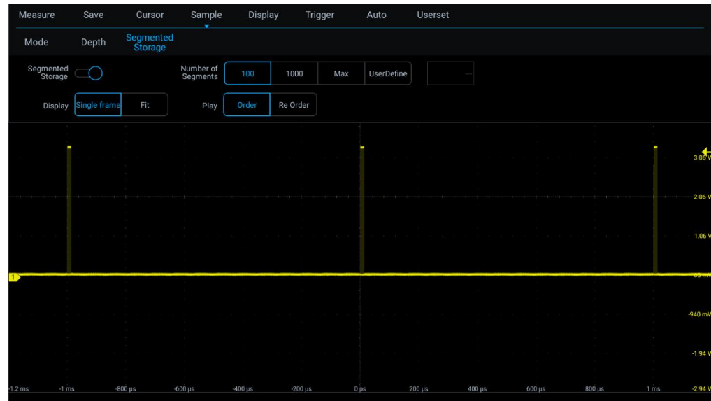
Figure 11-11 Segmented storage waveform acquisition
