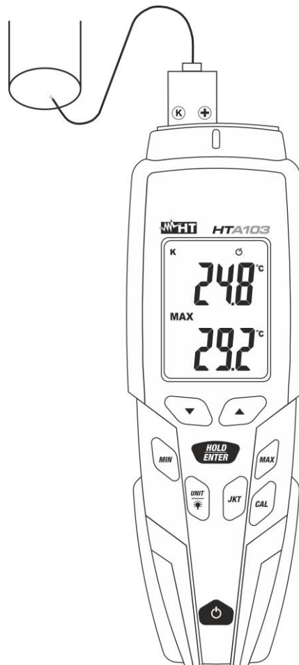
Fig. 5: Use of the instrument for temperature measurement
