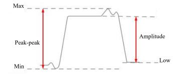
Figure 6-5 Voltage Measurement
