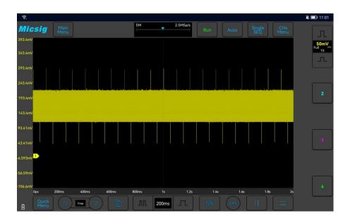
Figure 5-3 Abnormal Signal in Periodic Signals
