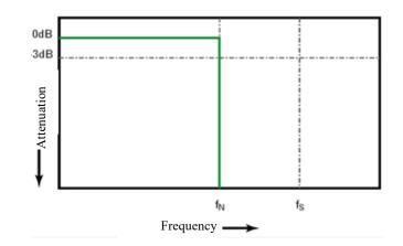
Figure 10-2 Theoretical Brick-Wall Frequency Response
