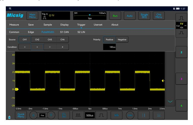
Figure 5-13 Pulse Width Trigger Setting Menu
