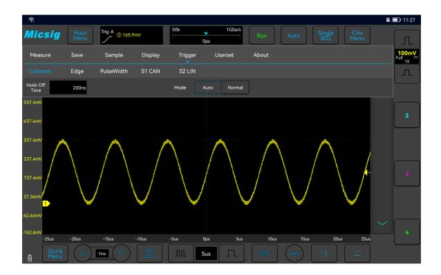
Figure 5-5 Oscilloscope Trigger Mode Setting
