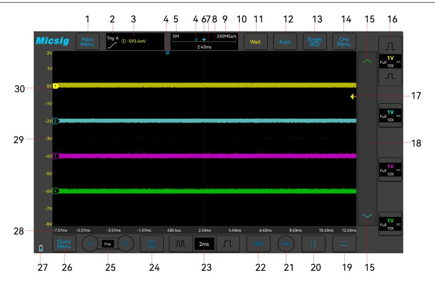
Figure 2-6 Oscilloscope Interface Display
