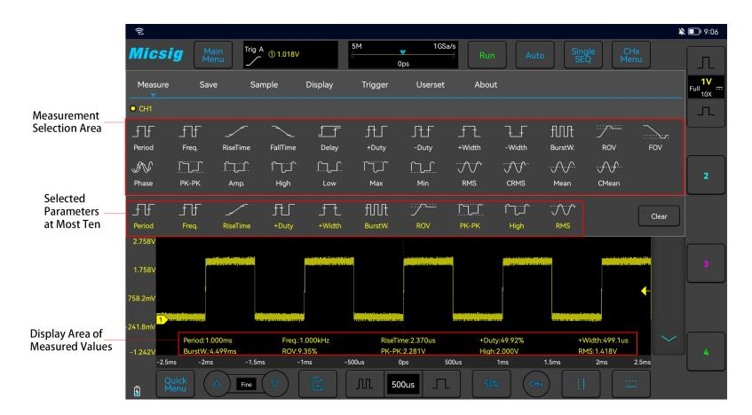
Figure 6-1 Automatic Measurement Menu
