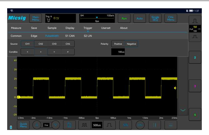
Figure 5-14 Negative Polarity Pulse Level Flip
