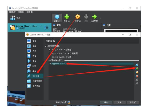
Figure 2-4 Setting USB device
