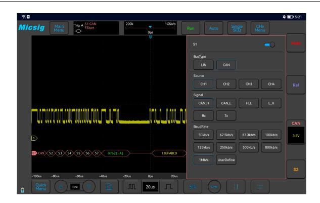
Figure 11-5 CAN Bus Configuration Menu
