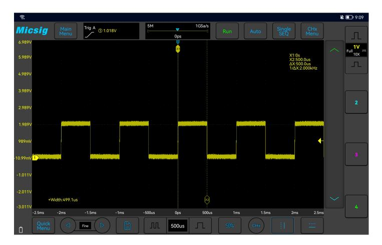
Figure 6-8 Cursor Measurement Pulse Width
