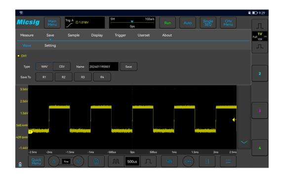
Figure 7-1 Save CH1 Reference Waveform Interface
