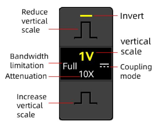
Figure 4-3 Channel Display Interface
