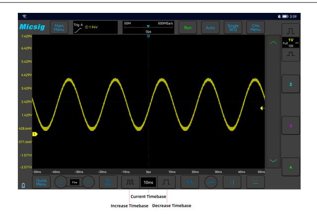
Figure 3-3 Adjust the Horizontal Time Base
