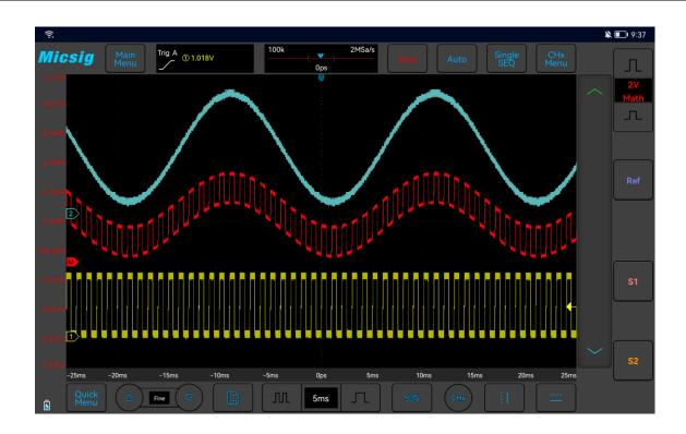
Figure 8-2 Mathematical Operation of CH1 adding CH2
