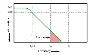
Figure 10-3 Sampling Rate and Oscilloscope Bandwidth
