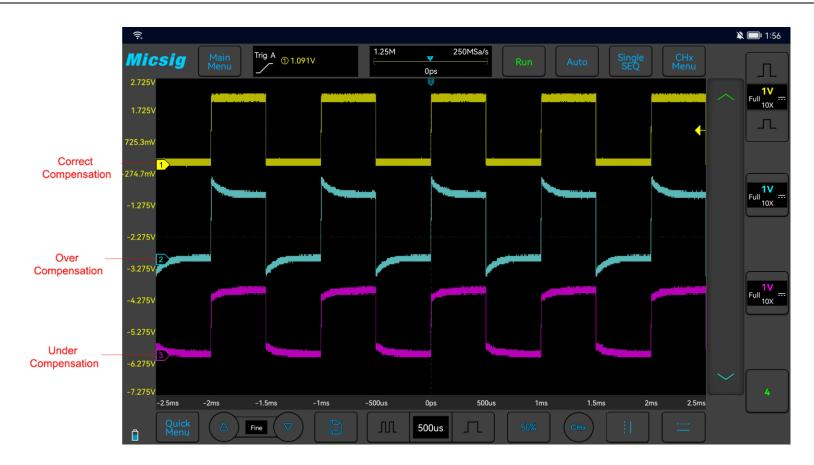
Figure 2-11 Probe Compensation
