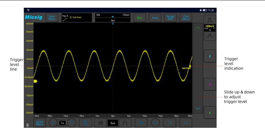
Figure 5-8 Trigger Level
