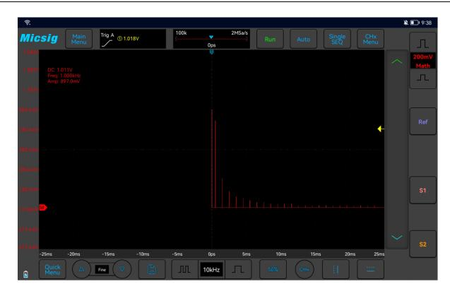
Figure 8-4 Spectrum Amplitude as V-Hz
