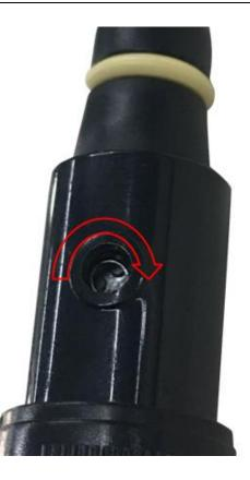
Figure 2-12 Probe Adjustment
