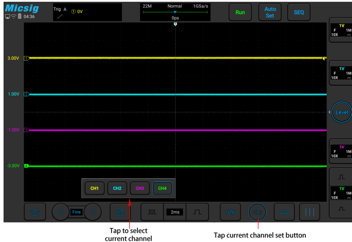
Figure 5-5 Using the Current Channel Selection Button
