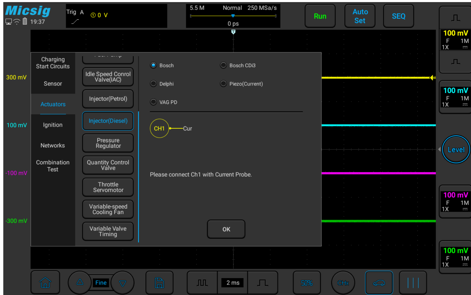
Figure 3-33 injector (diesel engine) test
