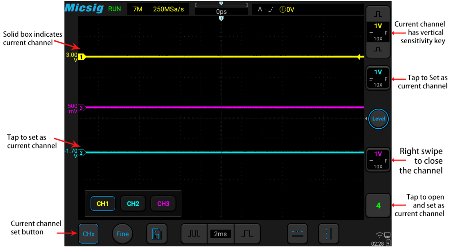
Figure 5-4 Channel Open, Close and Switching
