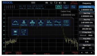
Advanced measurement mode provides test items required for the transmitter test such as multichannel power, ACP, and occupied BW.
