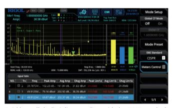
Quickly recall the limit line compliant with the CISPR standard (e.g. EN55011, EN55012, etc.) to carry out pre-test and monitor the target point with three different detectors.
