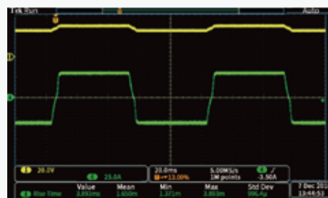
Control loop CC priority mode
