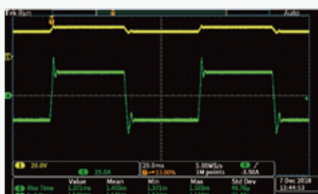
Control loop CV priority mode
