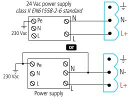
For transmitters with 100-240 Vac power supply:
