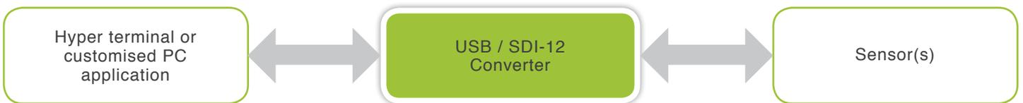
Figure 6 –TBS03 application; setup for SDI-12 tester mode
