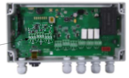
Example of MVA current/voltage board on a CA310 transmitter
