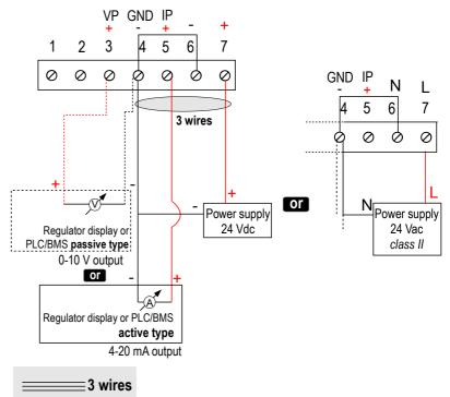
For  $\mbox{CP116-PO}$  and  $\mbox{CP116-PN}$  models with 4-20 mA output – passive :
