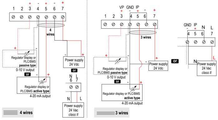
For CP112/113 - PO models and CP112/113 - PN models with 4-20 mA output - passive :
