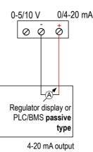
Connection of output in voltage 0-10 V :
