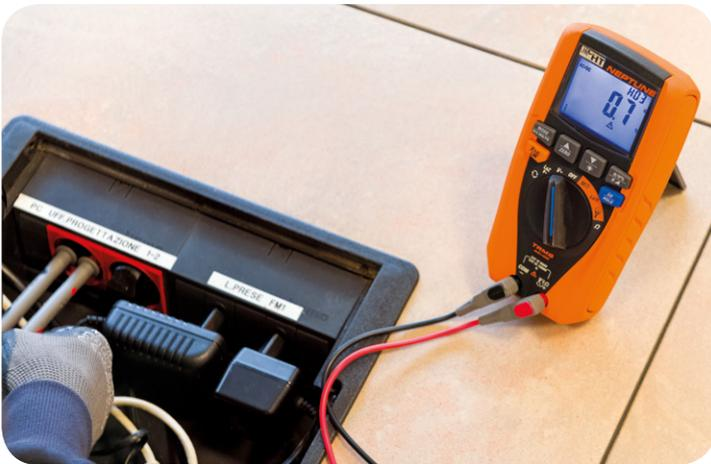
Measurement of **voltage harmonics**.
