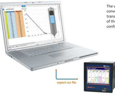
The value of every logical channel of MultiCon recorder may be converted using many various methods: by linear scaling, transfer with compliance to the user characteristics. In the case of the letter, each point of the characteristics required manual configuration, what extended the process significantly.
