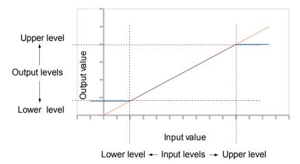
Fig. 7.88. Input (red)-output (blue) characteristic of signal in Current output module
