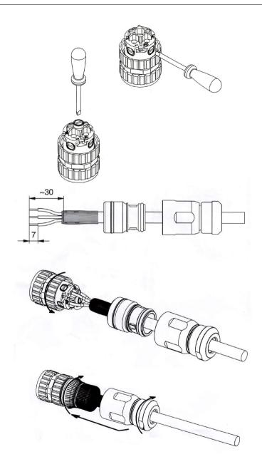
Fig. 8.15. Description of mounting ETH cable into IP67 connector
