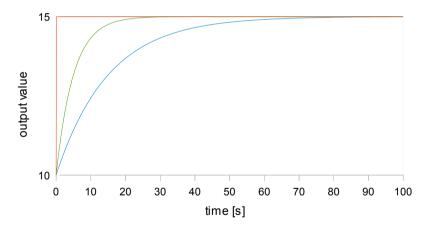
Fig. 7.37. Example of the input signal (red chart), filtered signal for the time constant = 5s (green chart) and the time constant = 15s (blue chart)
