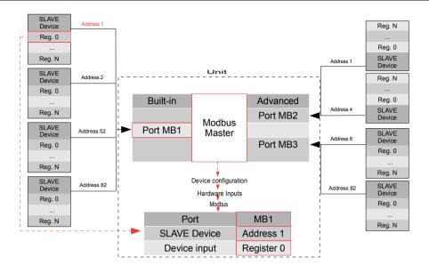
Fig. 7.49. An example of configuration block diagram of the Modbus protocol implemented in the device
