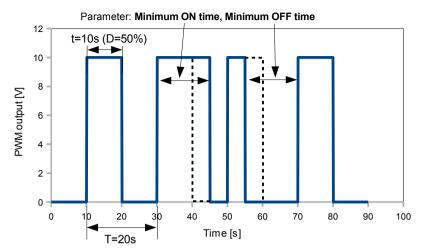
Fig. 7.86. Sample of output signal of OC-type relay in PULSE mode
