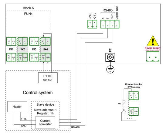
Fig. 7.110. The connection scheme for FUN4 hardware configuration in RTD mode and Modbus MB1 port
