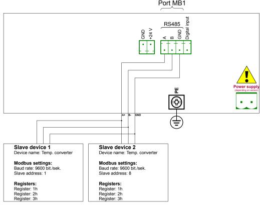
Fig. 7.128. Connection diagram for the Modbus port MB1
