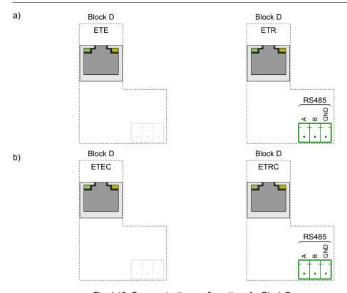
Fig. 4.12. Communication configurations for Block D
