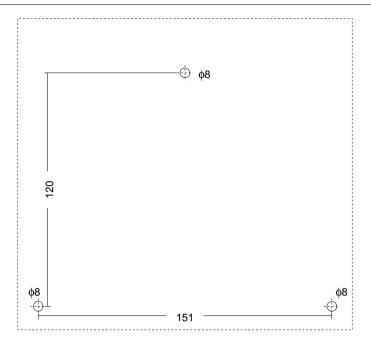
Fig. 4.2. Placement of the mounting holes
