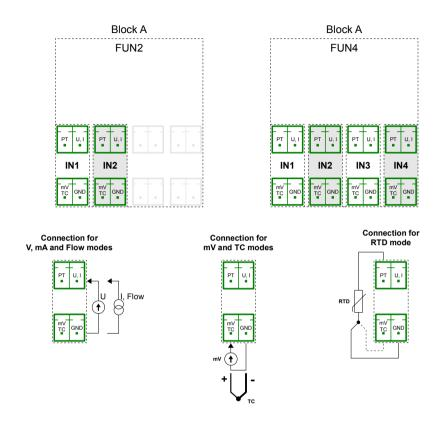
Fig. 8.2. Hardware input configurations for Block A
