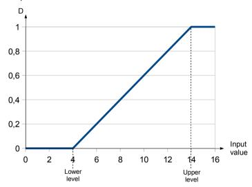
Fig. 7.85. Normalized duration ( $t_n$ ) of the output signal in PULSE mode for parameters: **Lower level=4**, **Upper level=14** (input signal lower than 4 has  $t_n$ =0, higher than 14 has  $t_n$ =1)
