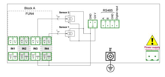
Fig. 8.5. Connections for 3 – wire sensor (current)
