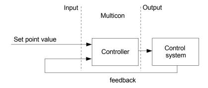
Fig. 7.56. The overall structure of control system implemented in the device
