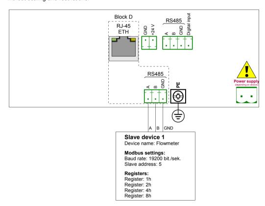
Fig. 7.96. Connection diagram for Modbus MB2
