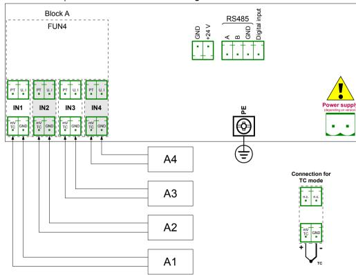
Fig. 7.64. Schematic diagram for the **FUN4** hardware configuration
