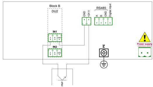
Fig. 7.72. DU2 hardware configuration and PNP type sensor connection scheme
