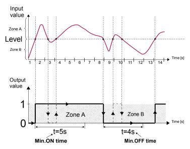
Fig. 7.83. Principle of relay output operation for sample timing settings: Min. ON time=5 sec., Min. OFF time=4 sec.
