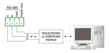
Fig. 4.13. Connection of RS-485 transmission signals
