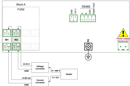
Fig. 7.58. Schematic diagram for the **FUN2** hardware configuration
