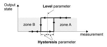
Fig. 7.79. One threshold control of the virtual relays
