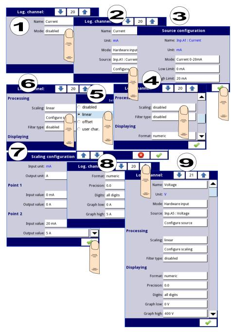
Fig. 7.59. Current and voltage source configuration example
