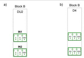
Fig. 8.7. Optoisolated hardware digital configurations for Block B
