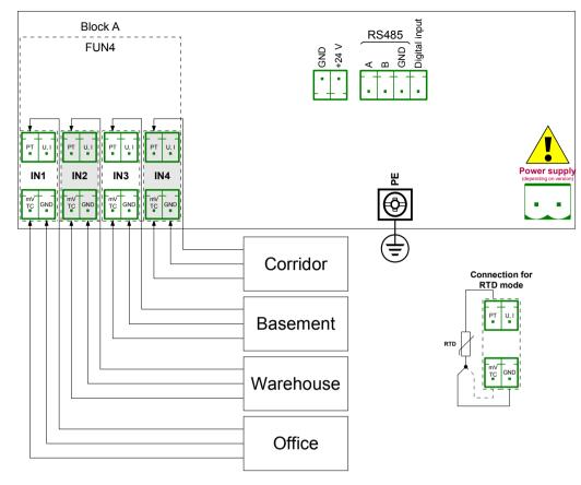
Fig. 7.66. Schematic diagram for the FUN4 hardware configuration
