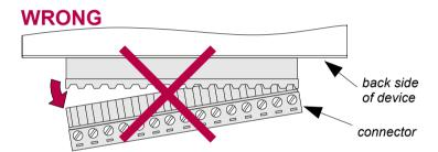
Fig. 4.3. Connectors removing method
