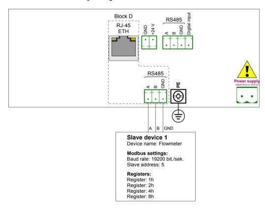
Fig. 7.129. Connection diagram for the Modbus MB2 port
