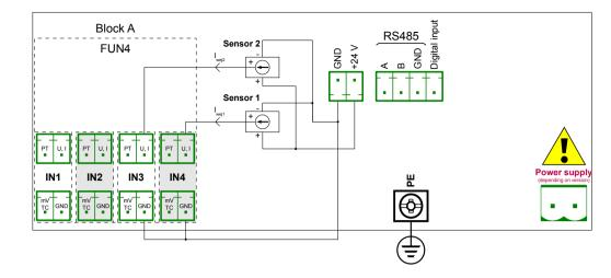
Fig. 8.6. Connections for 3 – wire sensor (voltage)
