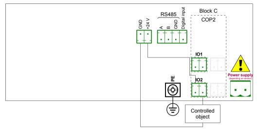
Fig. 7.91. Passive current output connection example
