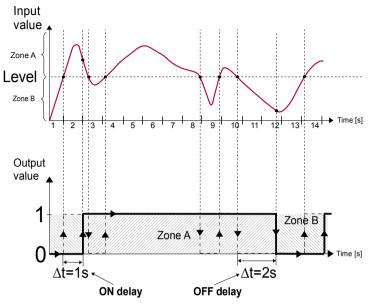
Fig. 7.82. Principle of virtual relay operation for sample timing settings:
