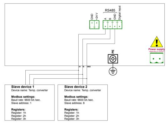
Fig. 7.68. Schematic diagram for SLAVE devices connected to MultiCon
