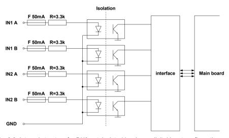
Fig. 8.8. Internal structure for DU2 optoisolated hardware digital input configuration
