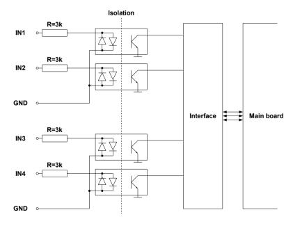
Fig. 8.9.Internal structure for D4 optoisolated hardware digital input configuration
