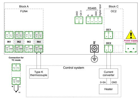
Fig. 7.111. The connection scheme for FUN4 hardware configuration in TC mode and OC2 hardware configuration
