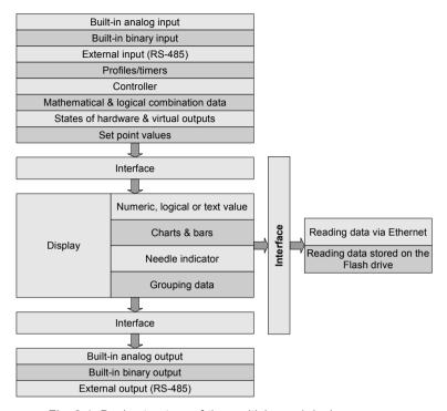
Fig. 2.1. Basic structure of the multichannel device
