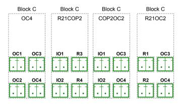
Fig. 8.12. Hardware output configurations for Block C
