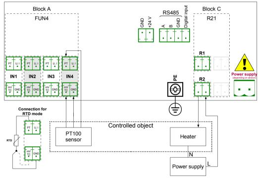
Fig. 7.90.Schematic diagram for the FUN4 hardware configuration in RTD mode and output hardware configuration
