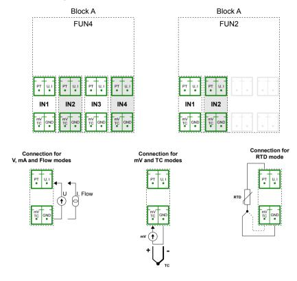
Fig. 4.9. Input configurations for Block A
