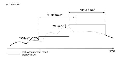
Fig. 7.38. Process of peak detection
