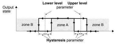
Fig. 7.80. Two threshold control of the virtual relays
