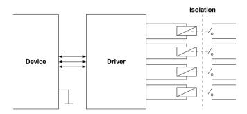
Fig. 8.13. Internal structure of the relay outputs hardware configurations
