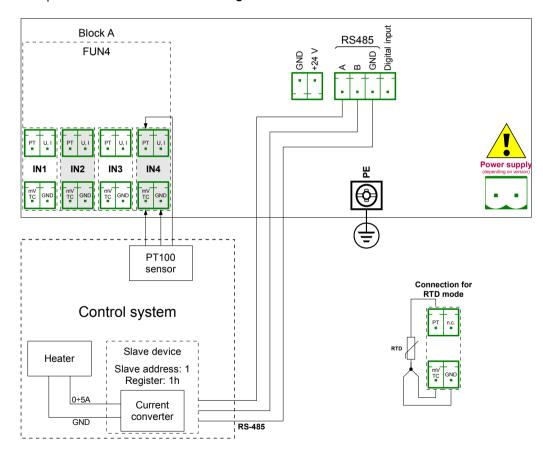
Fig. 7.70. Schematic diagram for the hardware configuration FUN4 and MB1 Modbus port
