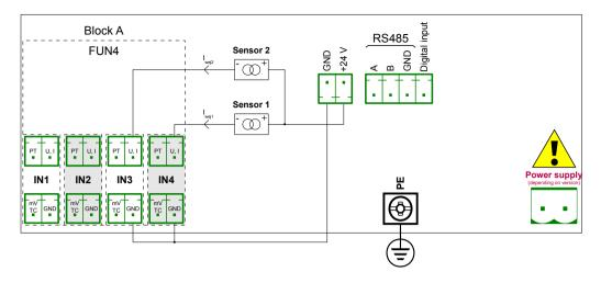
Fig. 8.4. Connections for 2 – wire sensor (current)
