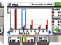
Power measurement: harmonics
