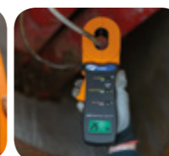
Earth resistance measurement with clamp T2100.
