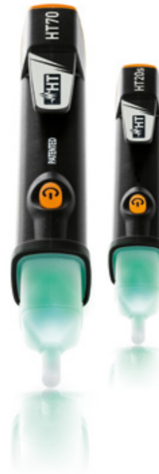
Step1 - Take HT70 and rest it on the assumed phase L1 of the three-phase system (on the conductor or sheath) for at least 5s and wait for the red LED to flash together with the buzzer sounding.
