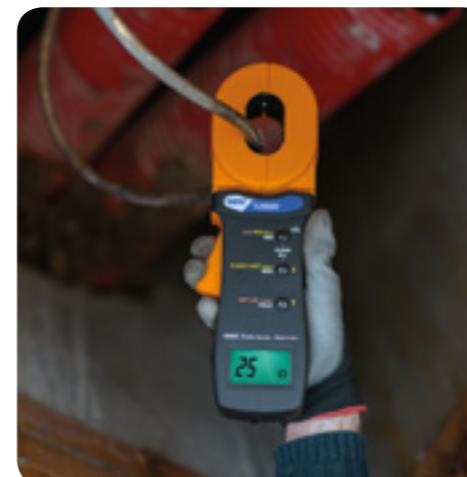
Measurement of earth resistance with Clamp T2100.
