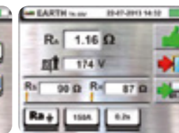
Earth resistance measurement result OK.
