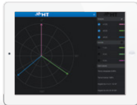
Voltage and current vector diagram.
