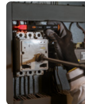
Step1 - Take HT70 and rest it on the assumed phase L1 of the three-phase system (on the conductor or sheath) for at least 5s and wait for the red LED to flash together with the buzzer sounding.
