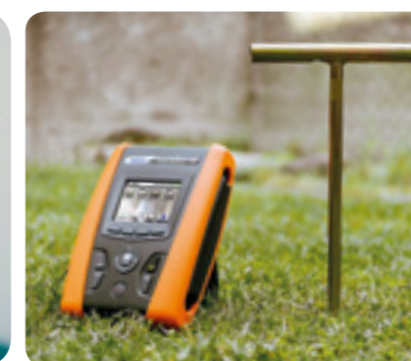
Measurement of earth impedance by voltammetric method
