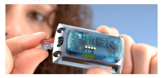
THE bestseller for transportation monitoring, fault diagnoses and load tests! The robust MSR 165 data logger is capable of taking 1600 acceleration (shock, vibrations) measurements per second in all three axes for up to five years.
