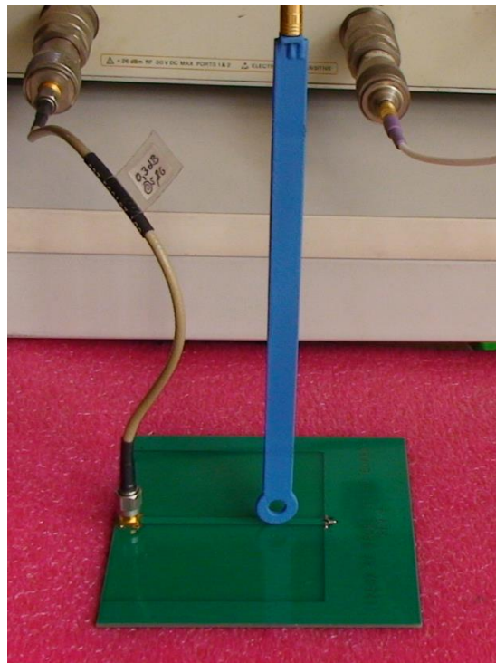
Picture 2 – measurement setup for coupling loss, 300kHz – 3GHz
