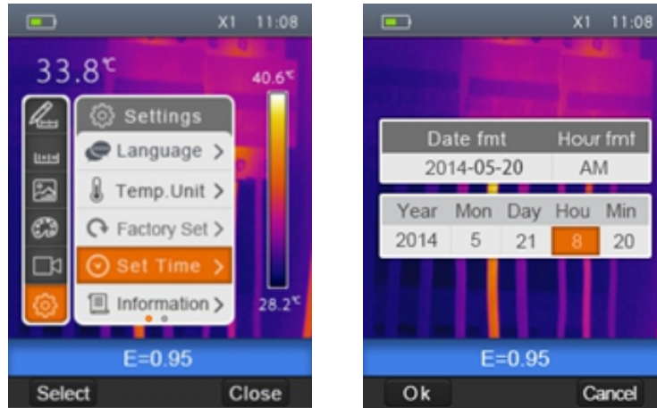
Fig. 11: Setting the instrument's date/time
