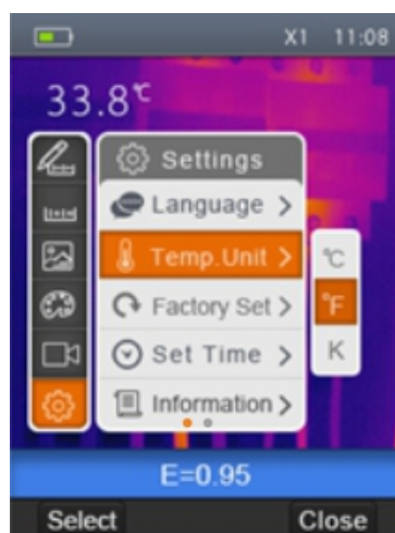
Fig. 9: Setting the temperature measuring unit
