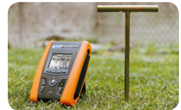
Earth resistance measurement by Volt-ampere method
