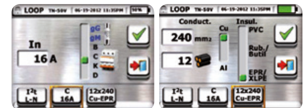
Setting of MCB/fuse type and rated current
