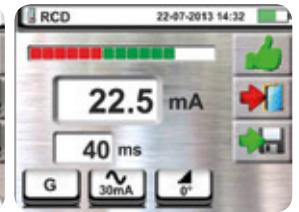
Ramp test result on RCD
